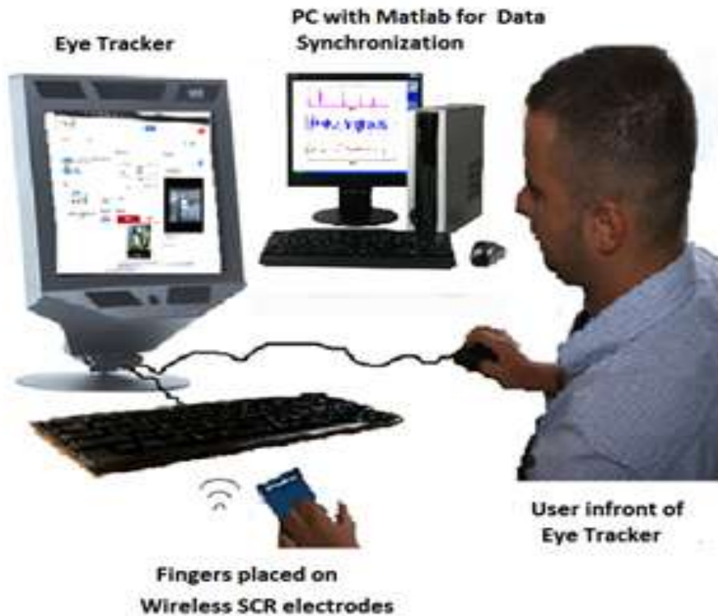
Fig.: User interaction with web pages on an eye tracker
